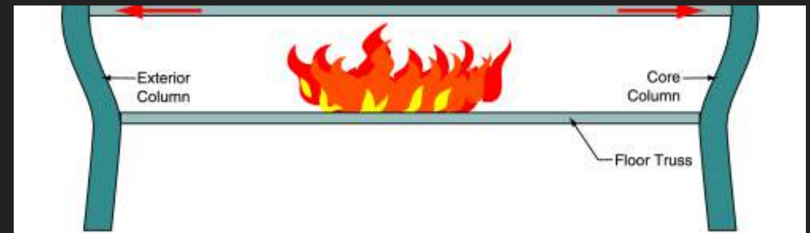
Figure 2-20 Expansion of floor slabs and framing results in outward deflection of columns and potential overload.
